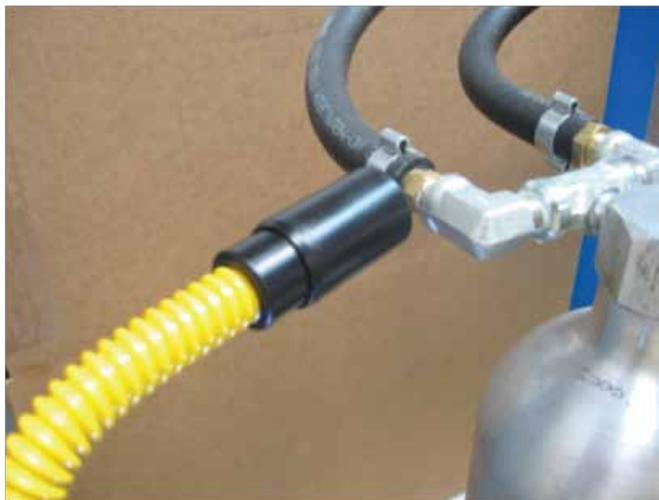
**Step 2.** Using the electronic leak detector go around the system to identify the leak site area. While moving the CO2 probe tip around the system it is best to keep the CO2 sensor face perpendicular to the surface being tested. **Note: If tip is bumped against the surface being tested the detector may momentarily go off, this false alert will go off right away. If the leak detector senses CO2 gas the alert will stay on for 10 to 40 seconds.**
