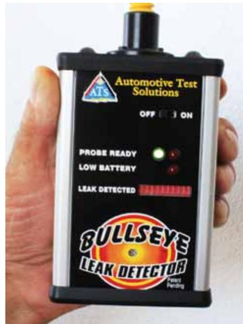
**Step 1.** Remove electronic leak detector from kit and turn on unit, allow unit to warm up the CO2 sensor tip. When unit is ready the red light will shut off and the green ready light will turn on, this will take about 90 seconds. For best results the leak detector CO2 sensor should be allowed to fully warm up for about 5 minutes.
