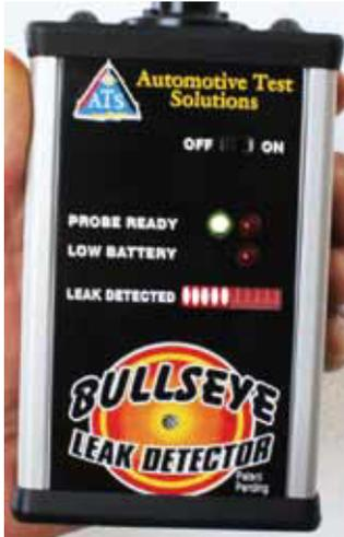
**Step 3.** When CO2 gas is detected the LED display bar is activated along with the audio alert (loud beeping noise). Once the detector has sensed CO2 the alerts will continue for about 10 to 40 seconds;
